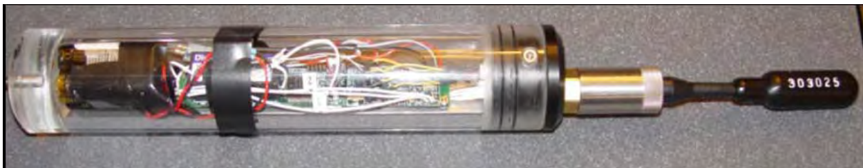
Figure 17. Autonomous Acoustic Recorder (AAR) instrument package for recording sounds, pressure, temperature, and inclination data to a 1-GB flash memory chip. The device can be powered by 4-AA batteries (Thode et al., 2006)
