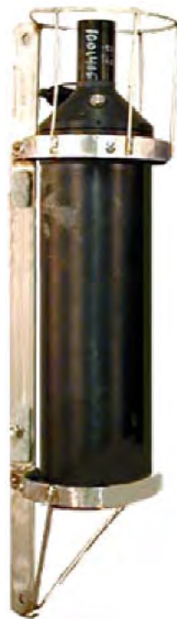
Figure 8. The PAL (Passive Acoustic Listener) in a deployment case (Nystuen, 2006).
