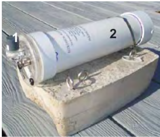
Figure 9. The EAR (Ecological Acoustic Recorder) showing 1 – the hydrophone and 2 the housing attached to a dead weight (Lammers et. al., 2008).
