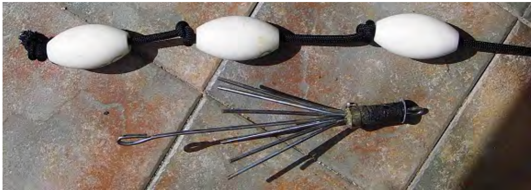
Figure 27. Theft of deployed PODs is a problem in some areas. One solution we have developed is the vertical grapple rig, that allows a deployment with no surface marker that can be retrieved without diving. The mooring is a weight with the POD and a line with a few small pressure-resistant floats, such as those used on the headline of gill nets to hold it up to above around half the water depth at low tide (Retrieved from http://www.chelonia.co.uk/vertical_grapple.htm , see Figure 28).
