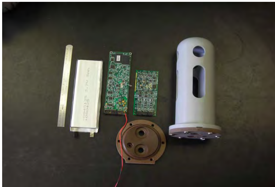
Figure 10. The DMON (Digital Acoustic Monitor) (DMON flyer, A. Bocconcelli, personal communication, October 17, 2009; Johnson, unpublished).
